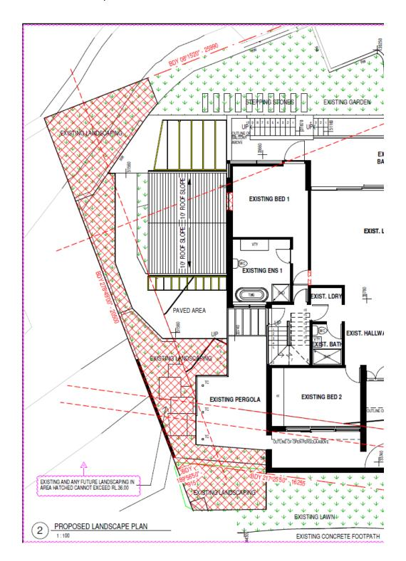
c) The pergola to the north-east and south-west sides of the carer's rooms are to be open, except for a maximum depth of 300mm to allow for weather-proofing.
